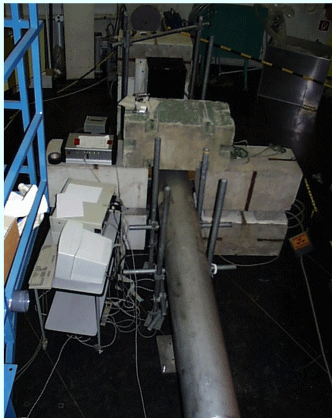
Dedicated radial flight tube at old FRM Munich - shielding incomplete
